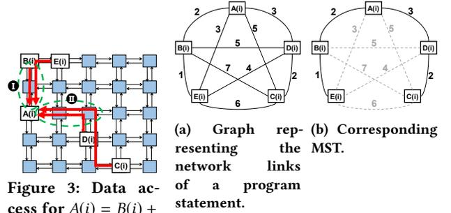
Figure 3: Data access for  $A(i) = B(i) + C(i) + D(i) + E(i)$ .
