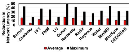
Figure 19: Reduction in on-chip network latencies (simulation results).
