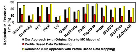
Figure 23: Comparison against a profile-based data mapping scheme.
