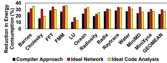
Figure 24: Reduction in energy compared to default computation placement (simulation results).
