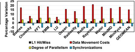
Figure 18: Contribution of different metrics to the execution time (simulation results).
