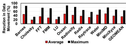
Figure 13: Data movement reduction over the original applications.
