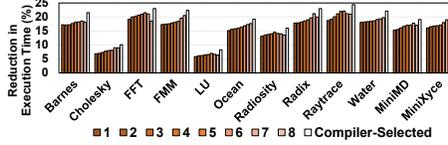
Figure 20: Results with different statement window sizes. 1-8 correspond to fixed window sizes for entire application.
